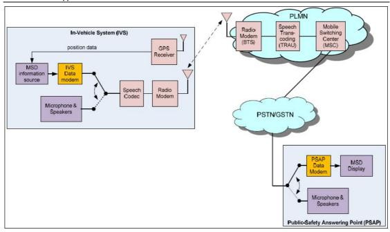
When triggered by a request from the PSAP operator through the PSAP modem, the in-band IVS data modem is used to transmit the relevant information (MSD) through the voice path established to the PSAP. Transmitting the MSD information through this voice path enables the system to use the E112 routing protocols deployed in existing networks.
