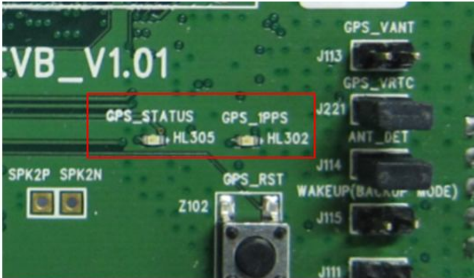
Figure 11: GNSS LED Indicator
